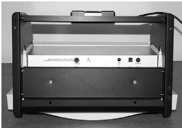
7. Connect the power cable and USB cable to the bottom of the digitizer.
